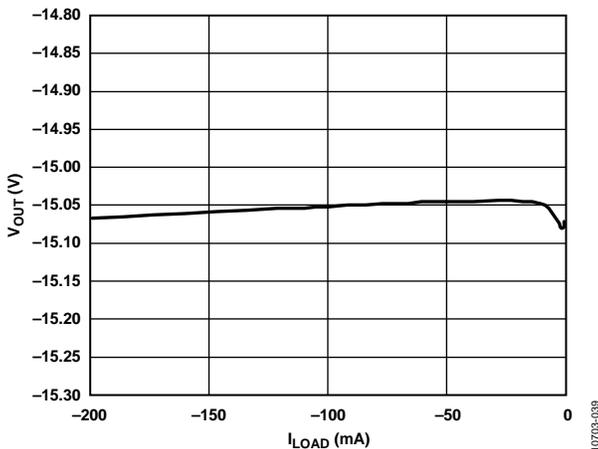
Figure 41. Output Voltage ( $V_{OUT}$ ) vs. Load Current ( $I_{LOAD}$ ), Adjustable Output Voltage,  $V_{OUT} = -15\text{ V}$
