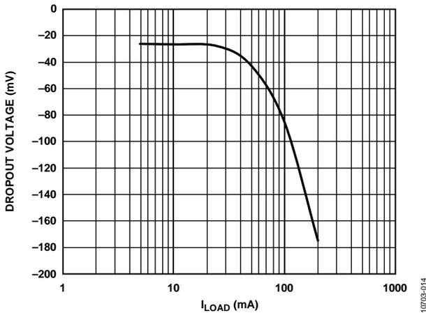
Figure 16. Dropout Voltage vs. Load Current (ILOAD)
