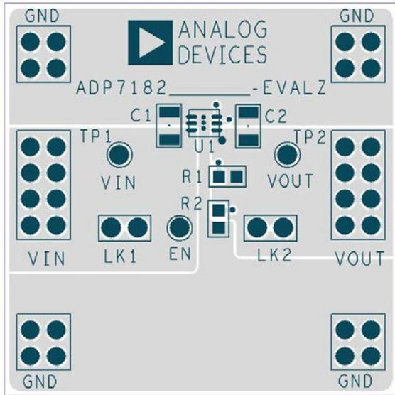
Figure 101. Example of the 6-Lead LFCSP PCB Layout
