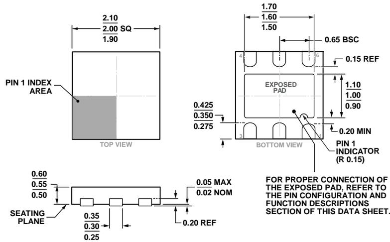
Figure 104. 6-Lead Lead Frame Chip Scale Package [LFCSP\_UD]
