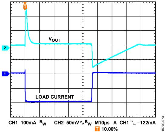
Figure 75. Load Transient Response,  $V_{OUT} = -5\text{ V}$ ,  $I_{LOAD} = -1\text{ mA}$  to  $-200\text{ mA}$ ,
