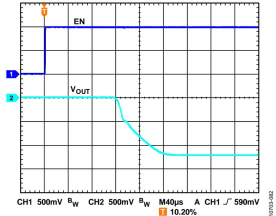
Figure 84. Typical Start-Up Behavior, Positive Going Enable
