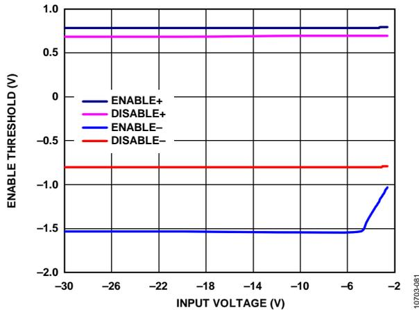
Figure 83. Typical EN Pin Thresholds vs. Input Voltage
