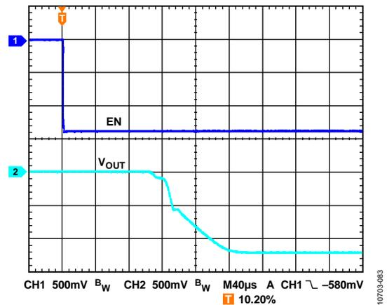
Figure 85. Typical Start-Up Behavior, Negative Going Enable
