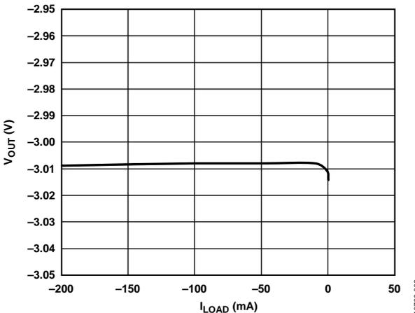
Figure 10. Output Voltage ( $V_{OUT}$ ) vs. Load Current ( $I_{LOAD}$ )
