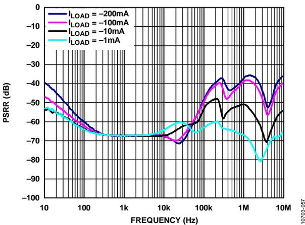
Figure 59. Power Supply Rejection Ratio (PSRR) vs. Frequency, Adjustable Output Voltage,  $V_{OUT} = -15\text{ V}$  vs. Different Load Currents ( $I_{LOAD}$ ),  $V_{IN} = -16.5\text{ V}$  with Noise Reduction Network
