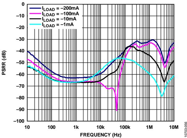
Figure 58. Power Supply Rejection Ratio (PSRR) vs. Frequency, Adjustable Output Voltage,  $V_{OUT} = -15\text{ V}$  vs. Different Load Currents ( $I_{LOAD}$ ),  $V_{IN} = -15.5\text{ V}$  with Noise Reduction Network
