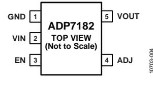
Figure 4. 5-Lead TSOT Pin Configuration, Adjustable Output Voltage
