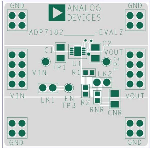
Figure 102. Example of the 8-Lead LFCSP PCB Layout
