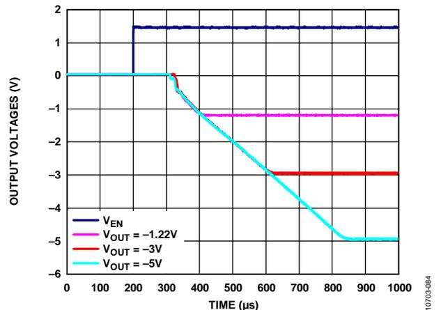
Figure 86. Typical Start-Up Behavior, Different Output Voltages
