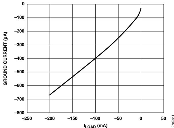
Figure 13. Ground Current vs. Load Current ( $I_{LOAD}$ )
