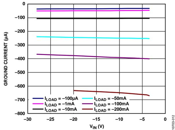
Figure 14. Ground Current vs. Input Voltage ( $V_{IN}$ )
