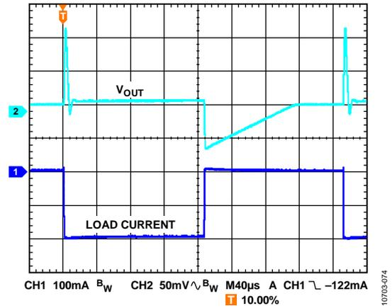
Figure 76. Load Transient Response,  $V_{OUT} = -15\text{ V}$ ,  $I_{LOAD} = -1\text{ mA}$  to  $-200\text{ mA}$ ,
