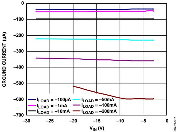
Figure 39. Ground Current vs. Input Voltage ( $V_{IN}$ ),  $V_{OUT} = -1.22\text{ V}$
