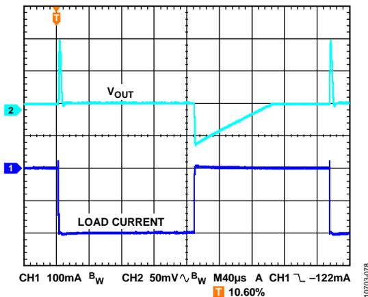
Figure 80. Output Transient Response,  $C_{OUT} = 2.2 \mu\text{F}$
