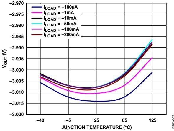
Figure 9. Output Voltage ( $V_{OUT}$ ) vs. Junction Temperature ( $T_j$ )
