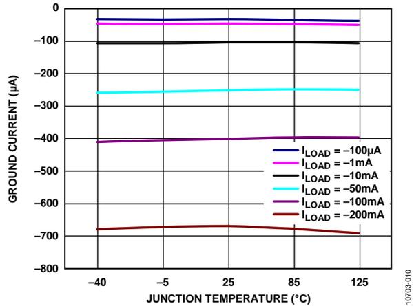
Figure 12. Ground Current vs. Junction Temperature ( $T_j$ )
