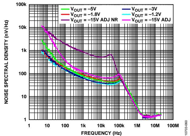
Figure 62. Noise Spectral Density, Various Output Voltages
