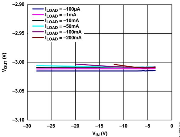
Figure 11. Output Voltage ( $V_{OUT}$ ) vs. Input Voltage ( $V_{IN}$ )
