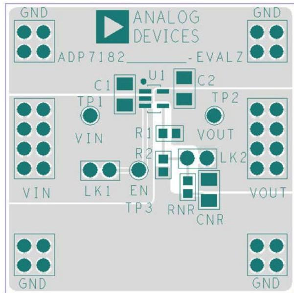
Figure 103. Example of the 5-Lead TSOT PCB Layout
