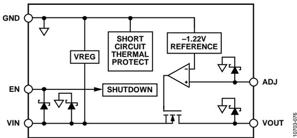
Figure 78. Adjustable Output Voltage Internal Block Diagram
