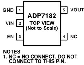
Figure 3. 5-Lead TSOT Pin Configuration, Fixed Output Voltage
