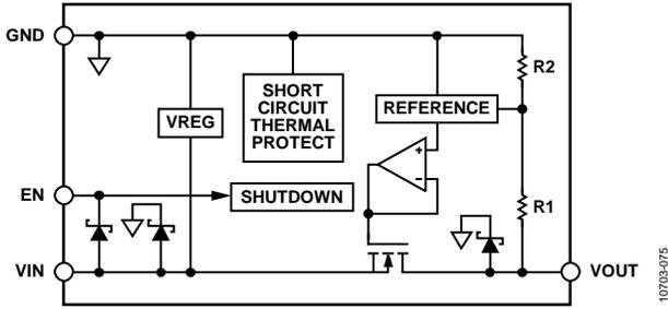
Figure 77. Fixed Output Voltage Internal Block Diagram
