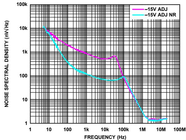
Figure 88.  $-15 \text{ V}$  Adjustable ADP7182 with and without the Noise Reduction Network ( $C_{NR}$  and  $R_{NR}$ )
